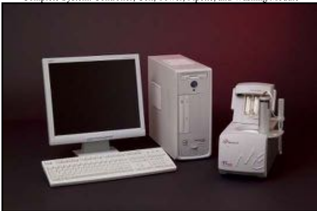
Complete System: Controller; Cell, Tower, Pipette, and Washing Module
