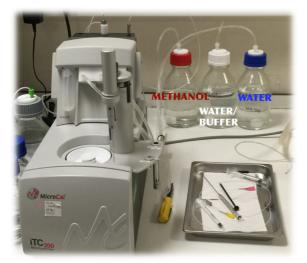
5) Start the run; the DP should be > 4.5 and the injection heats small. →
