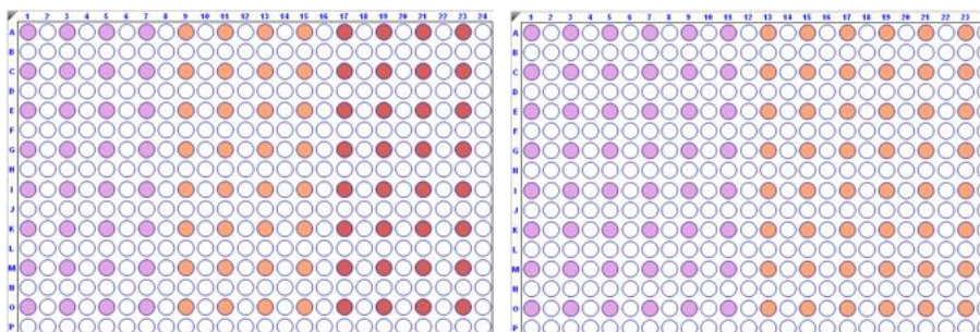
Figure 7-7: Biosensor Layout in 384-well Plates Using 32 (left) and 48 (right) Channels Read Head Setting.
