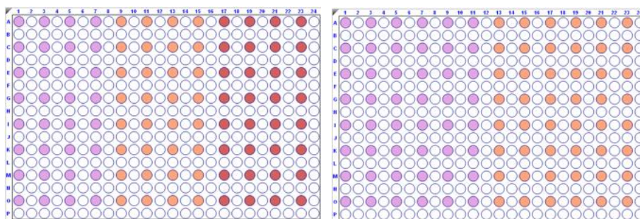
Figure 10-62: Biosensor Layout in 384-well Plates Using 32 (left) and 48 (right) Channels Read Head Setting.
